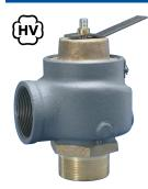
**Model 930** Extra high capacity for industrial, commercial and residential low pressure, steam heating boilers. Cast iron with bronze nozzle, disc and guide. Large seat area/guide area ratio, along with disc pivot design insures top valve performance. Flat bronze valve seats are lapped for optimum performance. Reversible lift lever for "pull-up" or "pull-down" manual testing.
