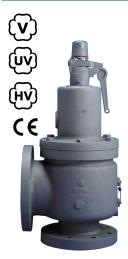
**Models 6252 and 6254** Heavy duty construction of high quality cast iron with stainless steel semi-nozzle trim. Bolted bonnet design for easy maintenance. Seats lapped to optical flatness. Dual control rings offer easy adjustability for precision opening with minimum pre-open or simmer and exact blowdown control. Heavy duty lift lever assembly.
